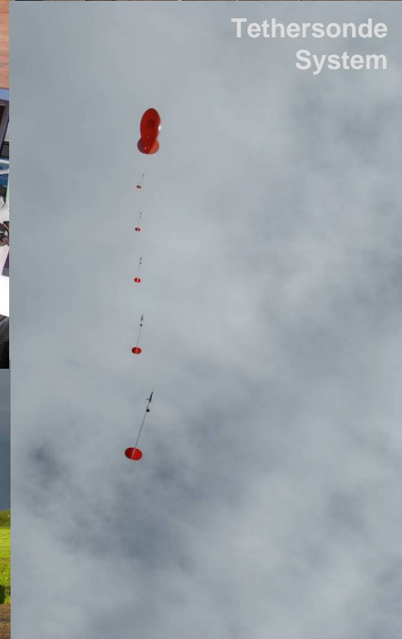
AMMOS (Automated Mobile Meteorological Observation System)
