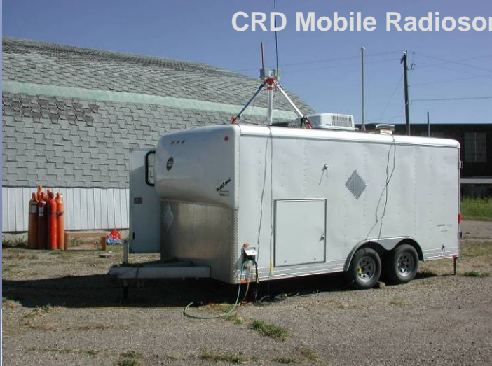
ATMOS (Automated Transportable Meteorological Observation System)
