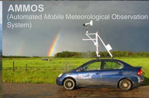
ATMOS (Automated Transportable Meteorological Observation System)
